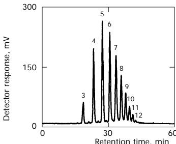
Separation of dextrane oligomers with 3–12 glucose units using column packed with polar porous polymer beads in hydrophilic interaction HPLC
